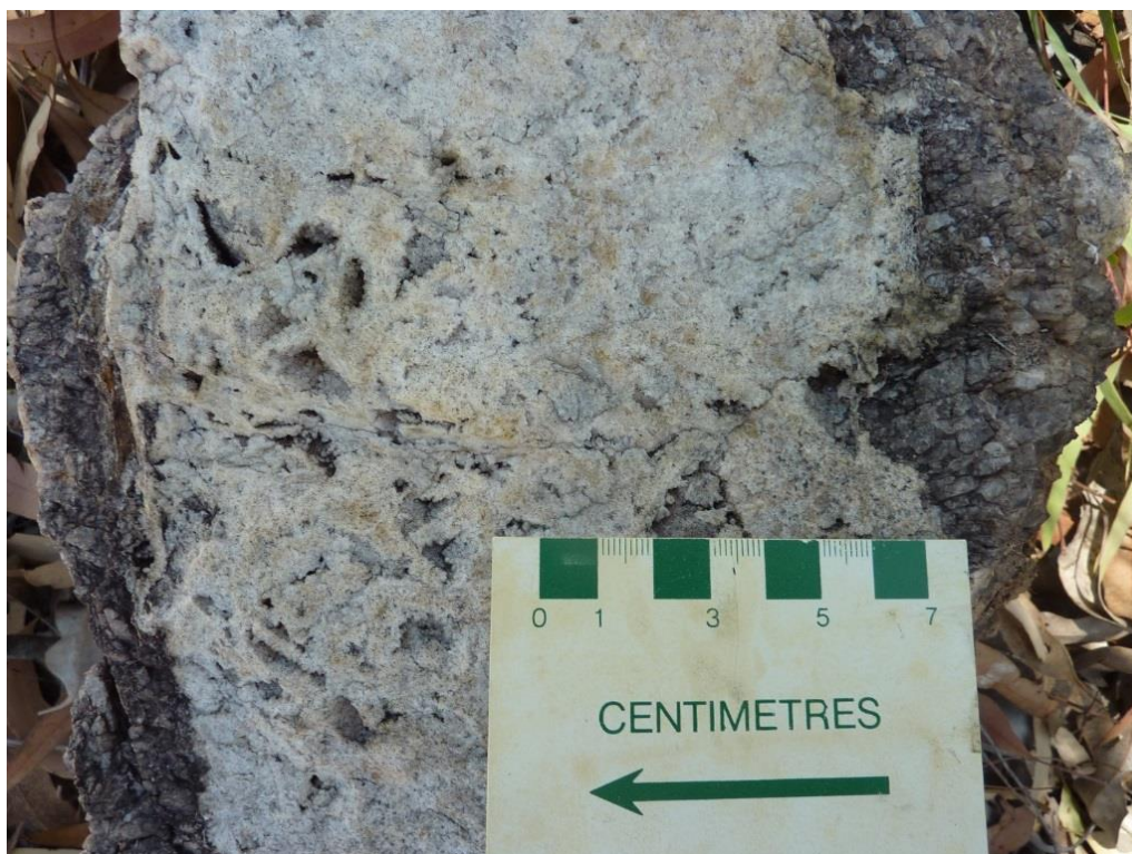
Figure 11: Platy, lattice textured quartz with fluorite along vein selvage at Perseverance Lode, Fluorspar Group workings
